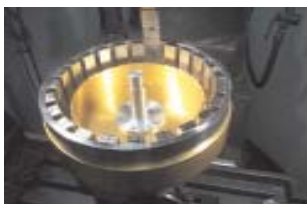
Figure 3: The final magnet being bonded in position
