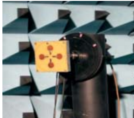
Antenna array under test in an anechoic chamber
